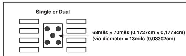
**Figure 14. PowerPAD PCB Etch and Via Pattern**
