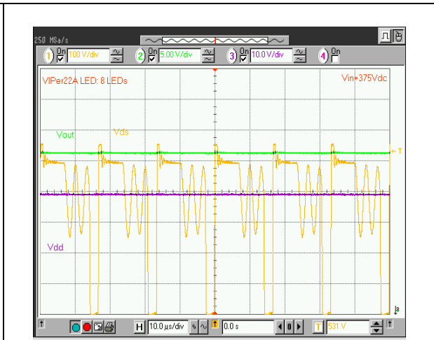
Figure 16. VIPer22A with 8 LEDs at output
