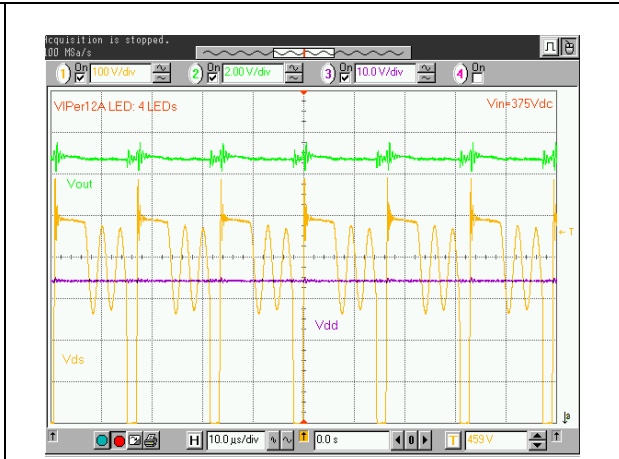
Figure 14. VIPer12A with 4 LEDs at output
