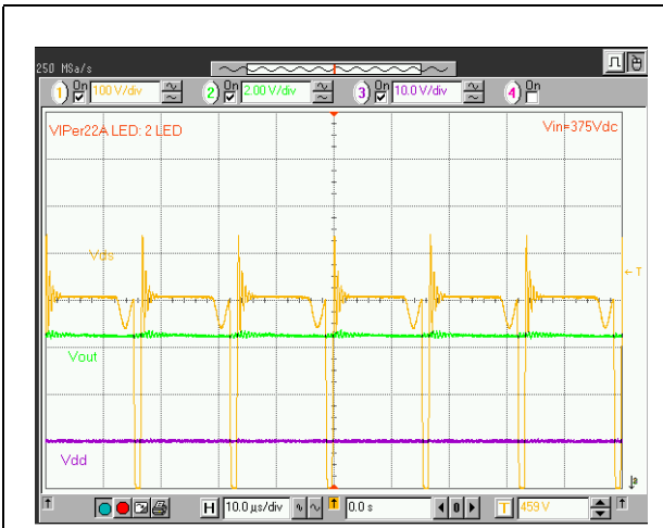
Figure 15. VIPer22A with 2 LEDs at output
