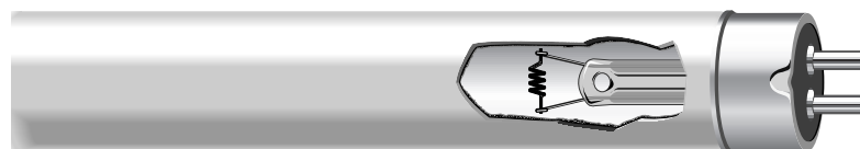
figure 1.2 lamp end with cold chamber – T5 and T5HO lamps
